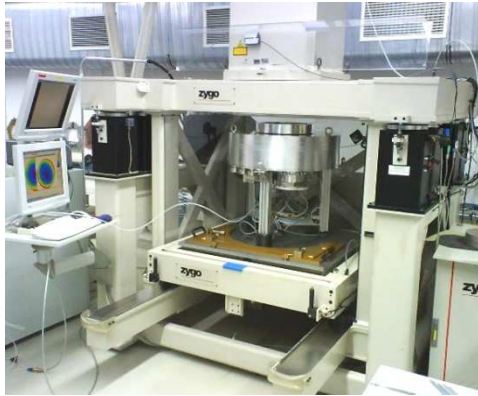
Figure 1: Zygo measurement set up with vacuum chamber and measurement data showing interferometric rings as a black and white pattern.
