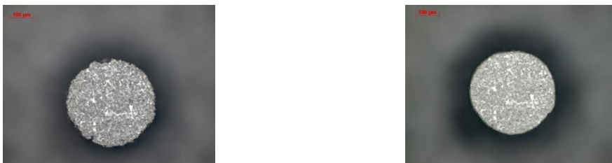
Figure 2: Left standard pins, right rounded pins. In both cases, the pin diameter is 400 µm.
