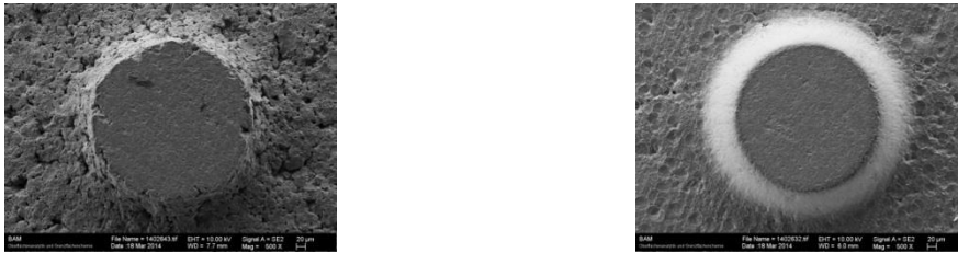
Figure 1: Different pin qualities: left standard pin, right advanced pin. In both cases, the pin diameter is 400 µm.
